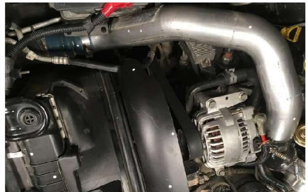
20. Install intake hose 2. Make sure the o-ring is all the way in, then tighten the two nuts on the bracket. After the bracket is tightened, push on the intake hose toward turbo as you tighten the clamp on turbo inlet. After tightened, make sure the o-ring is still seated tightly all the way in.
