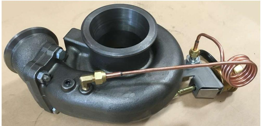
12. Before installing the turbine housing on your truck, rest the provided V-band clamp (F) on down pipe and factory clamp on exhaust pipe. Point the bolts as shown to make sure you have enough room to tighten them.
