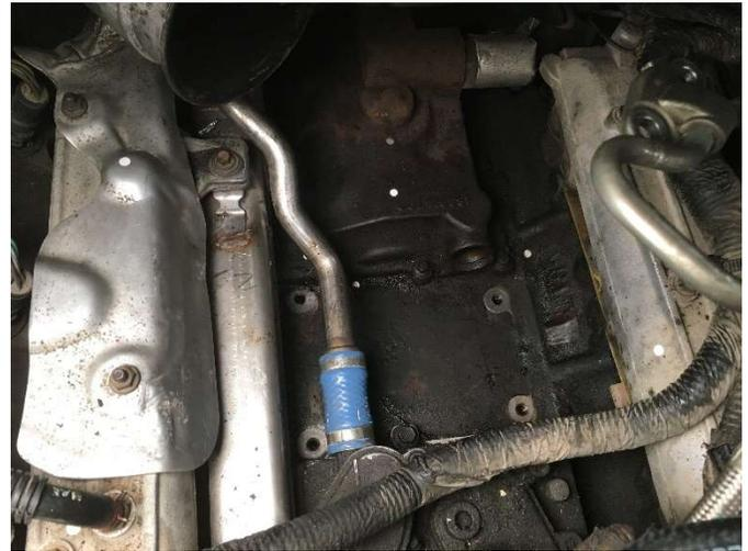
5. Make sure the o-rings are attached on both sides of oil drain tube (C) then tighten the worm gear clamp (S) onto the middle of the oil drain tube. Keep the clamp loose enough so that it can still move along the length of the oil drain tube. Insert the oil drain tube into the drain hole on the pedestal base (A). Make sure there is no debris in the drain hole of pedestal base. Blow it out if needed.
