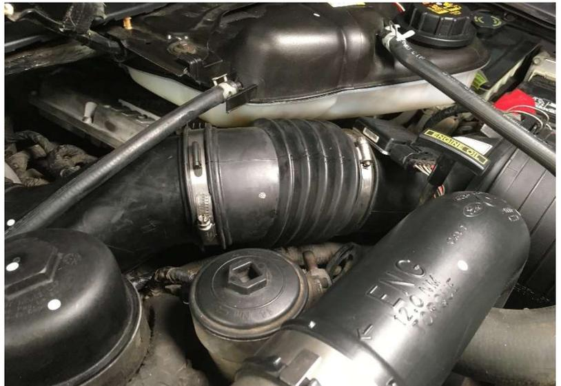
22. Remove all tools and parts from the engine bay. Start the truck and check for any oil leaks, air leaks, and vibration. If leaks are found, make sure all the clamps, bolts, or fittings are tight. Be sure that the oil pressure rises to the correct pressure. Allow it to idle for about 2-3 minutes without revving the engine. This allows the oil to reach the bearings of the new turbo. Do not allow truck to idle for long periods of time, especially on new turbo because it may cause turbo leaks.
